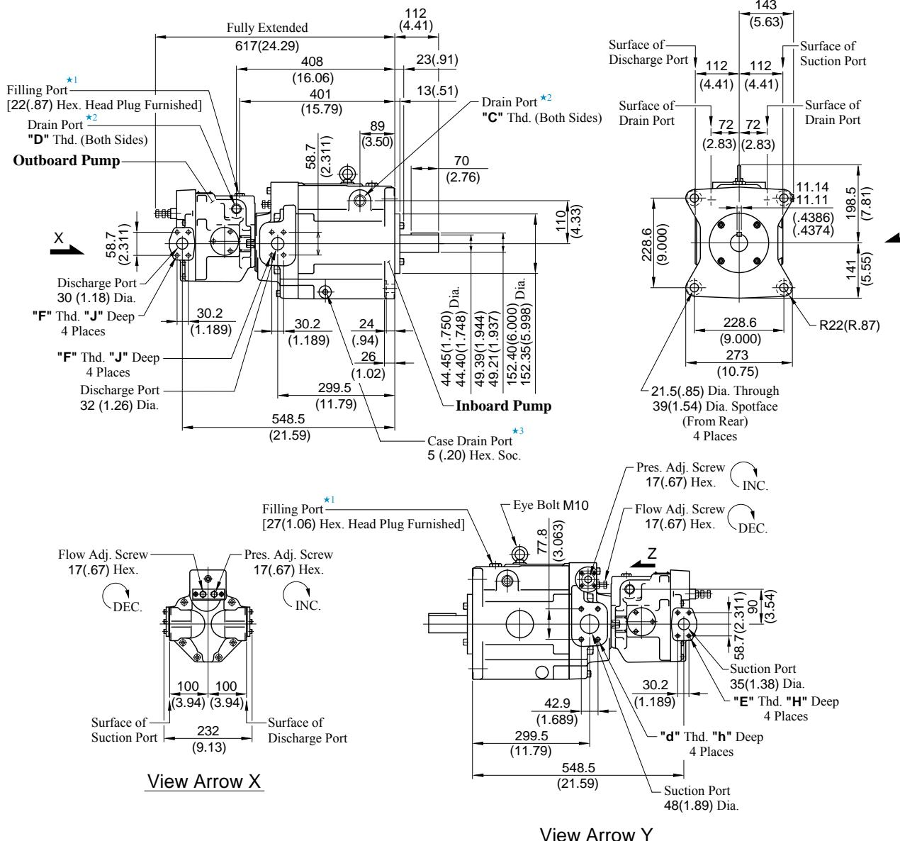
★1. Install the pump so that the "Filling Port" is at the top.
