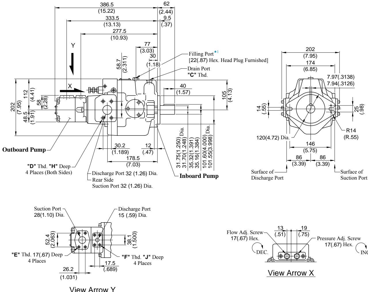
★ 1. Install the pump so that the "Filling Port" is at the top.
