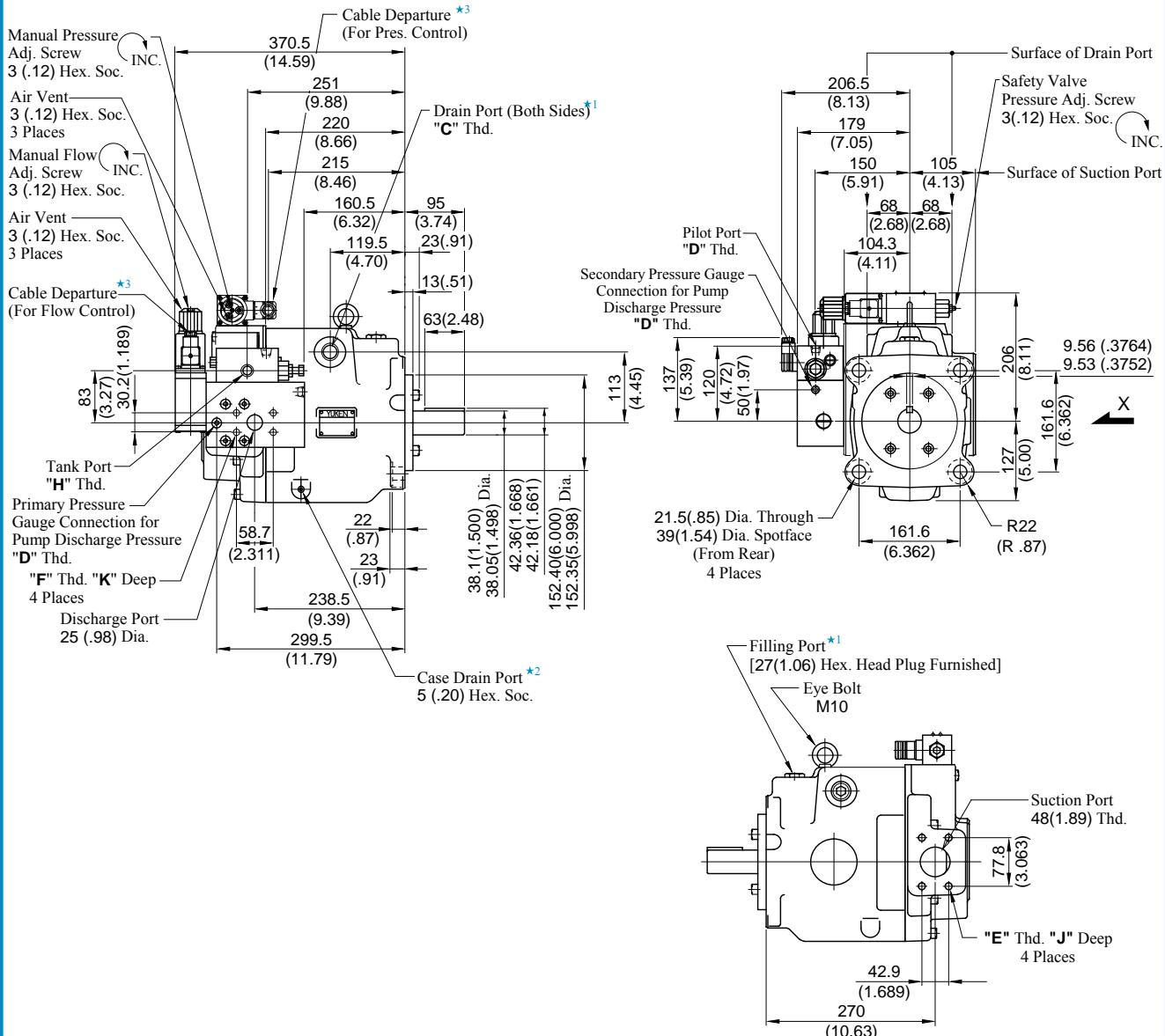
★ 1. Use either port of two pilot and drain ports at your option. Keep the remaining port plugged. Note that on the European Design Standard (6080 Design), only the left side, as viewed from the shaft end, of the drain port is machined.
