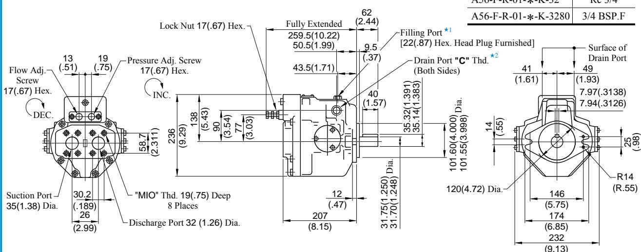
★1. Install the pump so that the "Filling Port" is at the top.
