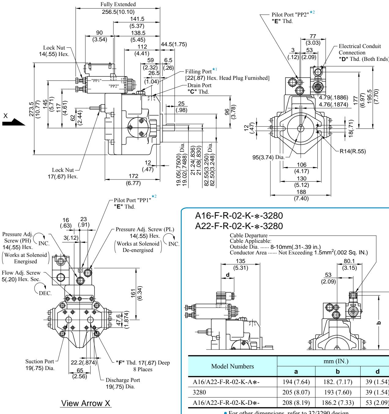
★ 1. Install the pump so that the "Filling Port" is at the top.
