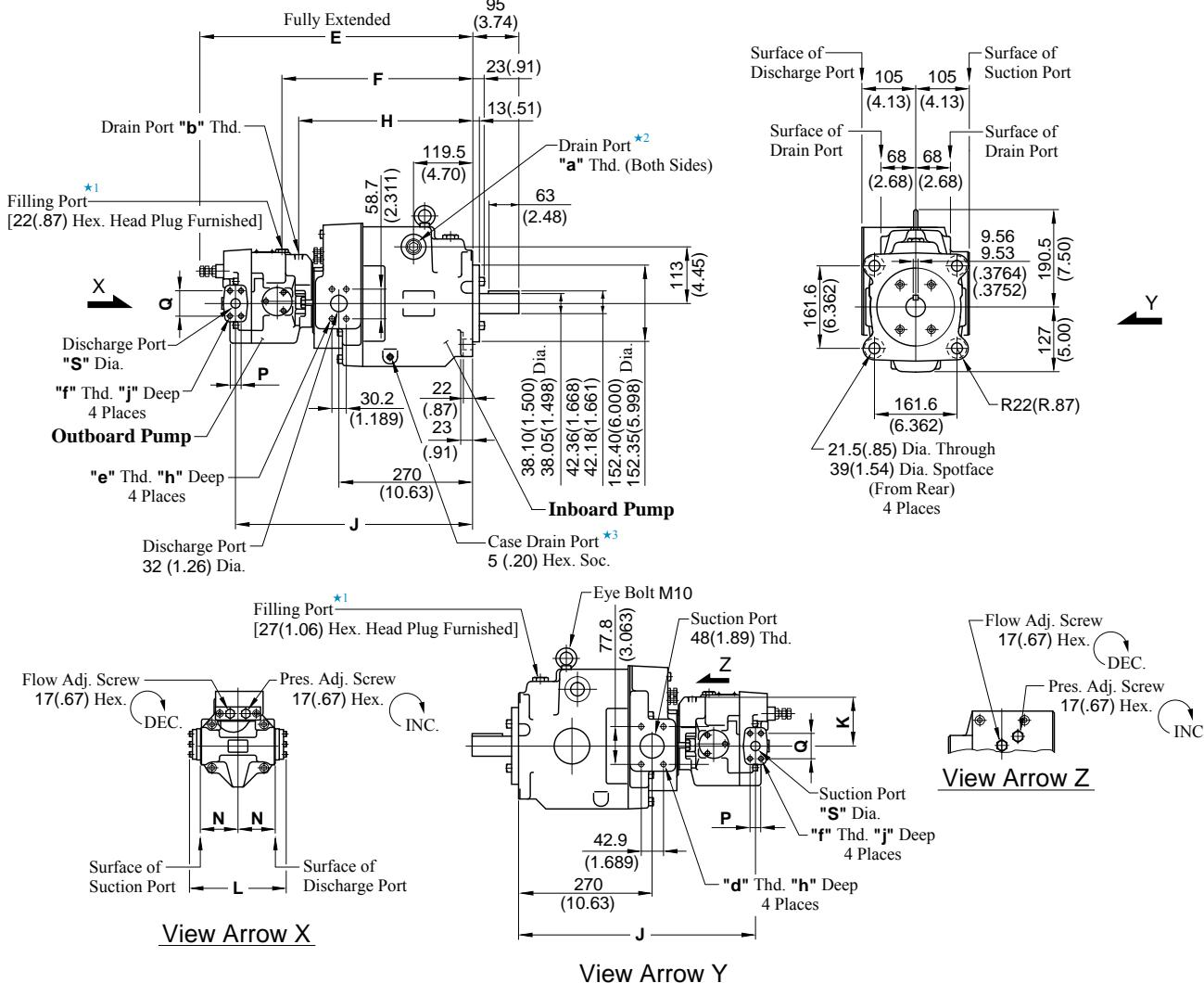
★1. Install the pump so that the "Filling Port" is at the top.
