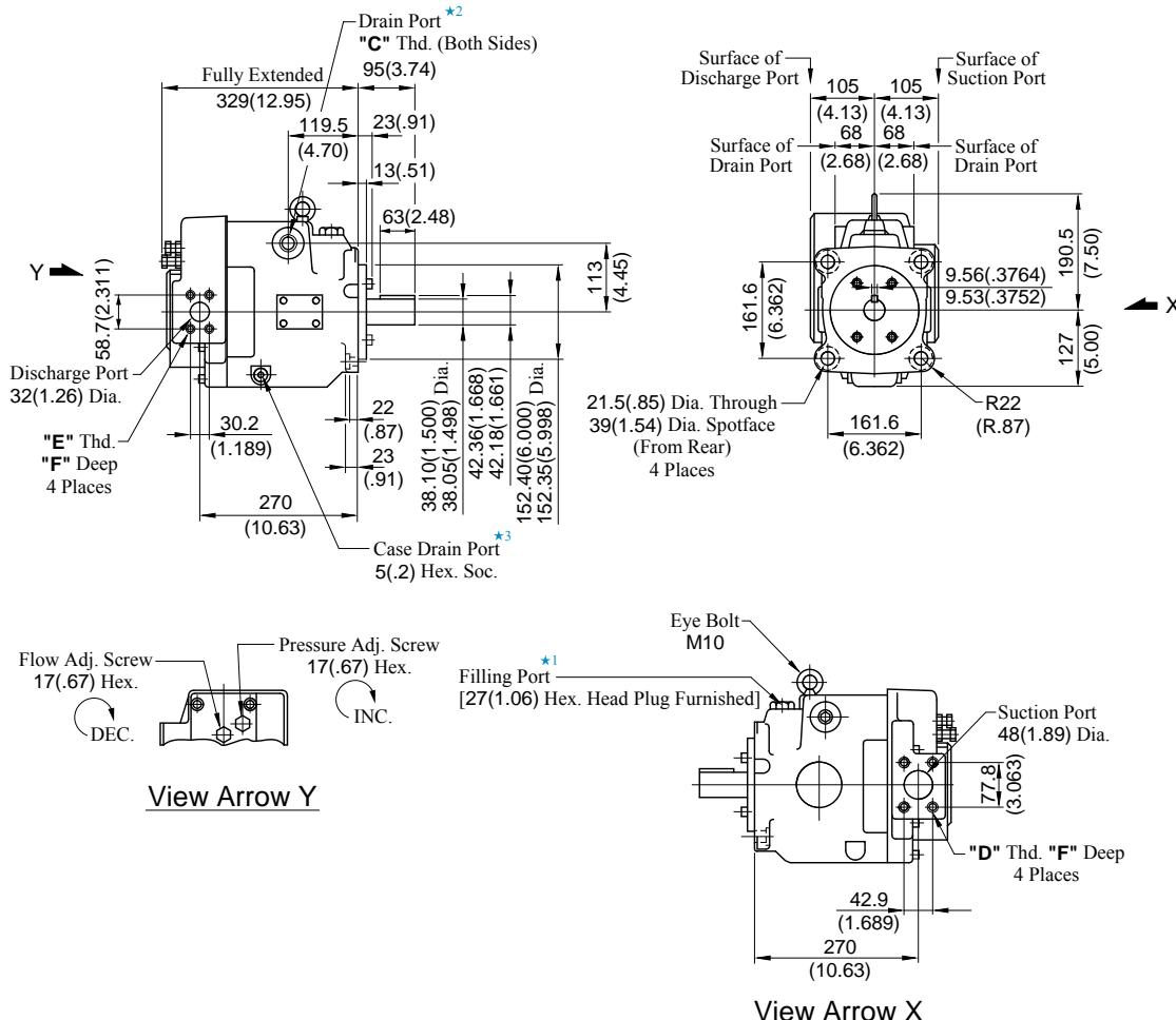
★ 1. Install the pump so that the "Filling Port" is at the top.
