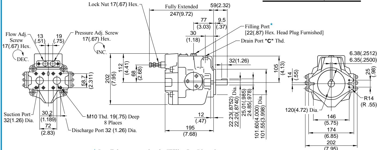
★ Install the pump so that the "Filling Port" is at the top.
