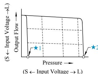
★1. Unloading pressure when input signal is 0 V.
