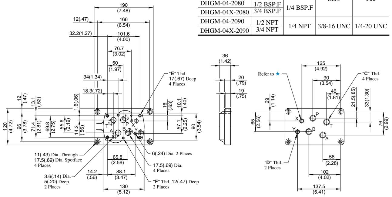
★ Used only on external pilot type valves. To be plugged on internal pilot type valves.
